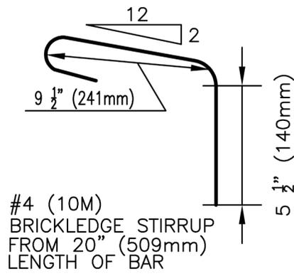
Reinforcing steel can now be added to help support the brick that will be installed later in the construction process. The steel needed to accomplish the reinforcing
