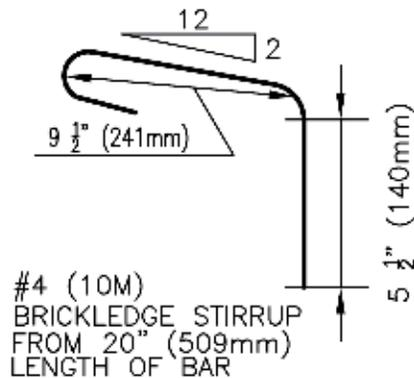
Reinforcing steel can now be added to help support the brick that will be installed later in the construction process. The steel needed to accomplish the reinforcing
