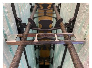
positioning locations which are 7/8" (22 mm) wide and a minimum of 1 3/8" (35 mm) long (length of holes varies depending on size of insert). This product is designed to ensure a minimum  $\frac{3}{4}$ " (19 mm) concrete coverage from the side of the foam, which is the minimum coverage as dictated by ACI regulations.
