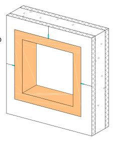
APPLY ENVIRO-DRI 3" MIN INTO ROUGH OPENING AND EXTERIOR FACE OF WALL AT SILL, JAMBS, HEAD
